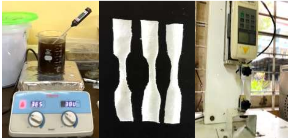
Figure 2. Equipment used for the preparation and tensile testing of polyester samples modified with coffee waste.
