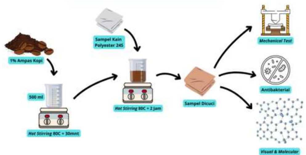
Figure 1. Flow diagram of the preparation and characterization of coffee waste–based polyester filtration media for drainage applications.
