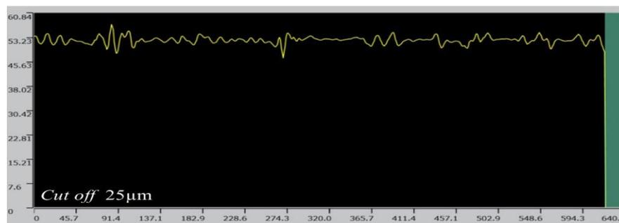
Figure 8. Representation measurement roughness-Ra using cutoff 25  $\mu\text{m}$
