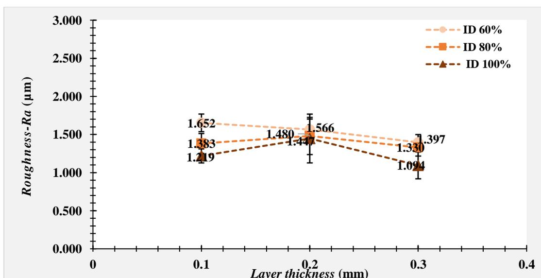
Figure 9. Graph of the results of the average roughness measurement-Ra at the top point surface using a cutoff of 25  $\mu\text{m}$
