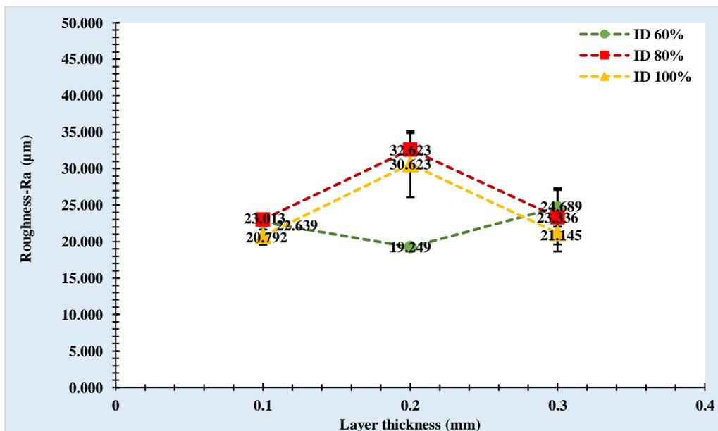
Figure 7. Graph of the results of the average roughness measurement-Ra at the bottom point surface using a cutoff of  $800\ \mu\text{m}$
