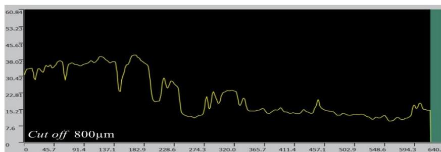
Figure 5. Representation measurement roughness-Ra using cutoff 800  $\mu\text{m}$
