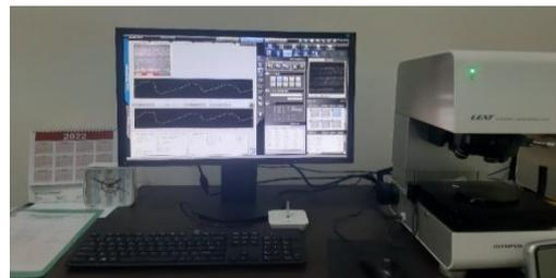
Figure 3. Laser-scanning confocal digital microscope (LEXT OLS4100)
