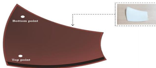
Figure 4. Roughness measurement points on the propeller blade
