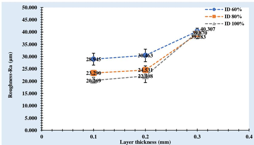
Figure 6. Graph of the results of the average roughness measurement-Ra at the top point surface using a cutoff of  $800\ \mu\text{m}$
