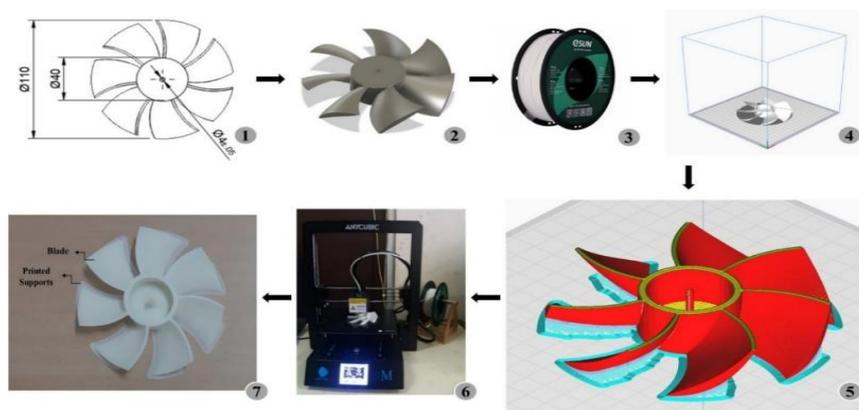
Figure. 2 The steps to produce propeller (Dimensional 3D, STL, Material PLA, Transfer file to slicer Ultimaker Cura, Parameters setup, Build product geometry; Printed product)
