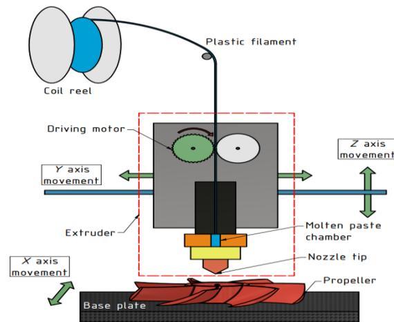
Figure. 1 Schematic of the FDM process
