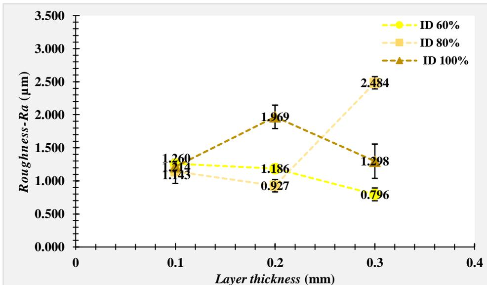
Figure 10. Graph of the results of the average roughness measurement-Ra at the bottom point surface using a cutoff of 25 µm
