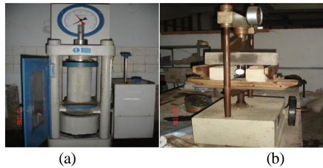
Figure 2. (a) Universal Testing Machine (b) Flexural Compressor Machine
