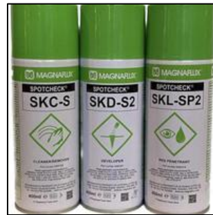
Figure 3. Set developer penetrant test
