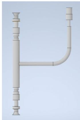
**Gambar 5.** Domain fluida check valve model 2
